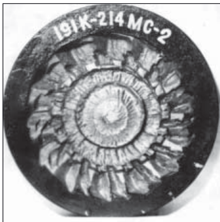
A 191K-214 MC-2 two-cone bit with a 3.7-mm difference in the pitch of the heel rows of the cones formed this metallic bottomhole pattern (Fig. 4).
