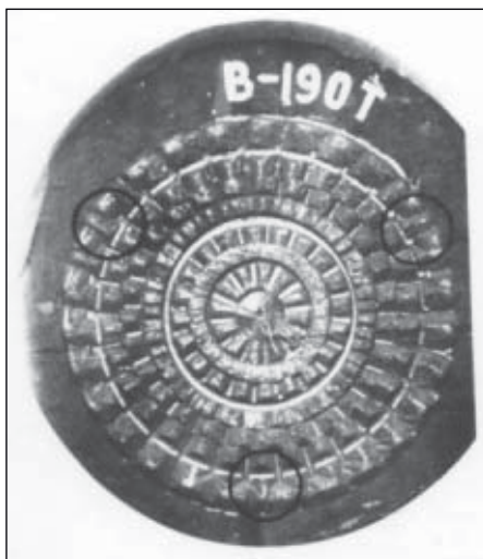
A commercial B-190T bit with varied pitch of the heel teeth in all cones rolled this steel bottom-hole pattern (Fig. 3).
