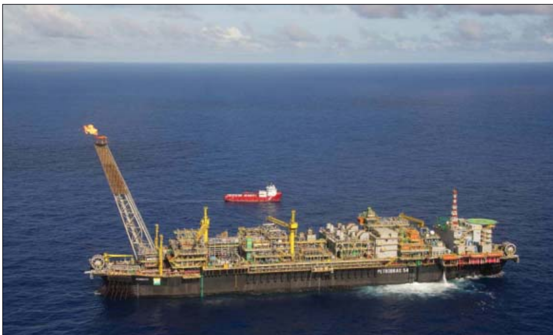
Petrobras expects the P-54 FPSO, installed in Roncador field off Brazil, to reach its 180,000 bo/d design capacity in second-half 2008 (Fig. 5). Photo from Petrobras.
